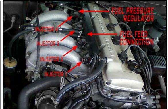
2. Use a 12mm socket wrench to remove the two primary M8 mounting bolts. Next, gently lift fuel rail up just enough to expose the 4 rubber fuel injector isolator cushions. They will either be stuck around the lower portion of the injector or still in the intake manifold injector ports. Also, find the 2 black plastic spacers found underneath each fuel rail tab. These pieces will not be reused.
